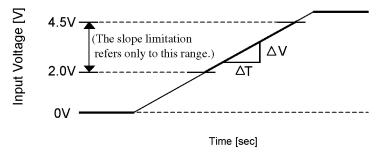
Slope:  $S = \Delta V / \Delta T$  [V/sec] S: 1V/20us to 1V/20ms
